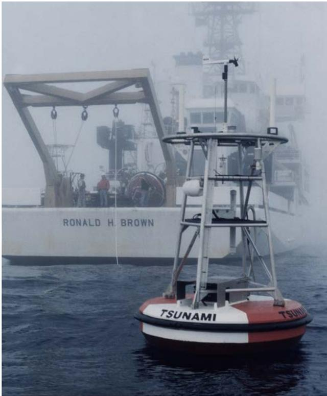
A DART buoy in the northern Pacific, near the Aleutian Islands, receives information from an instrument on the seafloor that calculates wave height. The buoy relays that information to satellites, which bounce it to regional warning centers.
